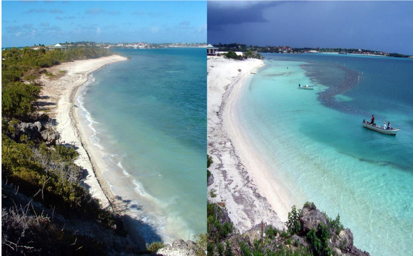
Artificial Reef off Maiden Island, Antigua. Note turbulent water and erosion ridges on beach before reef (left), and clear calm water after reef (right). COG, Dr. Alfredo Torruella
